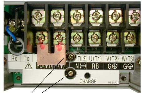
Retention screws for capacitor bank
