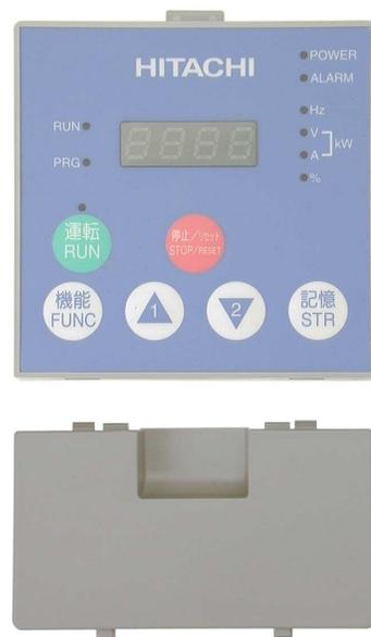
The digital operator / copy unit is optional, and occupies the entire keypad recess when mounted. It has the additional capability of reading (uploading) the parameter settings in the inverter into its memory. Then you can install the copy unit on another inverter and write (download) the parameter settings into that inverter. OEMs will find this unit particularly useful, as one can use a single copy unit to transfer parameter settings from one inverter to many.
