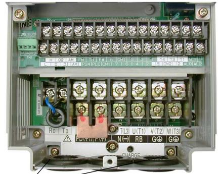
Retention screws for wire entry plate
